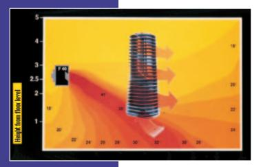
This results in the lower, hotter air being kept down by the higher, cooler air. Thus the different temperatures within the air-throw ensure a complete air mixing, thus reducing the temperature gradient between floor and ceiling.
